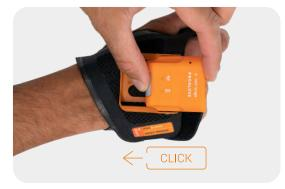
Insert the scanner in the Index Trigger.
