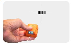
Press the button on the bottom of the Reel to trigger the scanner. Aim and scan barcode.
