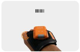
Press the textile trigger. Aim at the barcode and scan.
