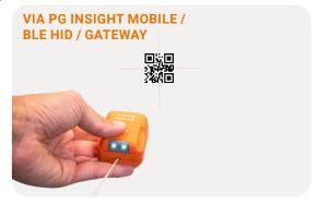
Press the trigger on the bottom of the Reel. Aim at the Pairing Barcode and scan.
