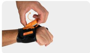
Use the fingers to press between scanner and the fastening rail of the Index Trigger. Press scanner up slightly and push it forward without scratching over the pins.
