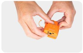
Use the fingers to press between scanner and the fastening rail of the Reel. Press scanner up slightly and push it forward.
