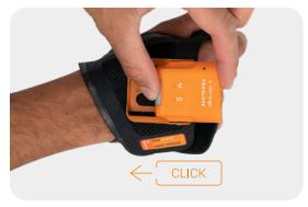
Insert the scanner in the Index Trigger.
